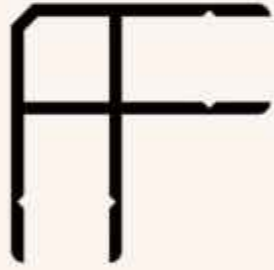
SIDING KENAR KAPAMA (SIDING EDGE CLOSURE)
